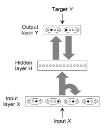
Figure 1. Network architecture. Large arrows stand for modifiable connections between fully connected layers. The input and output layers are made up of WTA clusters.
